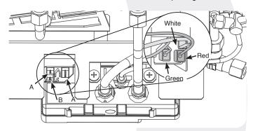
Replace with a new pilot assembly and check the spark gap.
