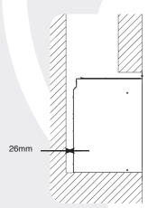
This appliance is not suitable for installation onto a combustible wall; all combustible materials must be removed from the area shown
