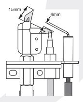
NOTE: Ensure the correct orientation when replacing.
