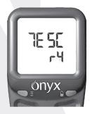
The handset is now at factory reset condition and a new pairing can be made.
