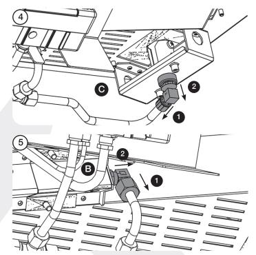
Turn on the gas supply and check for leaks.
